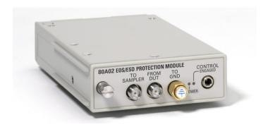
The 80A02 EOS/ESD Isolation module protects the sampling bridge of Tektronix DSA8300 <sup>1</sup> electrical sampling module inputs from damage due to electro-overstress (EOS) and electrostatic discharge (ESD) from circuit boards and cables. The 80A02 is for applications such as electrical TDR circuit board testing and cable testing where large static charges can be stored in the DUT.
